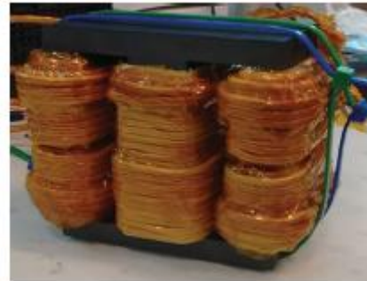
Fig. 9: 10kW/50kHz Three Port Transformer
